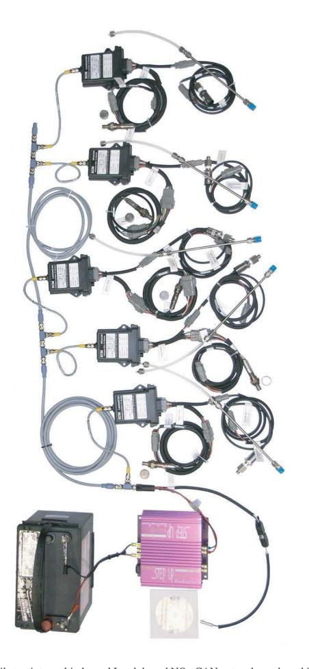
Easily tap into multi-channel Lambda and NOx CAN networks such as this.
